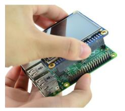
**NOTE:** The 4DPi-24-HAT is supported only by the 40 way header, and therefore pressing on the touch screen may result in the 4DPi-24-HAT moving towards the Raspberry Pi, and therefore the circuitry touching the Raspberry Pi. This could result in damage to either product if a short circuit were to occur. It is therefore highly encouraged to mount the display on the Pi using standoffs (not supplied)
