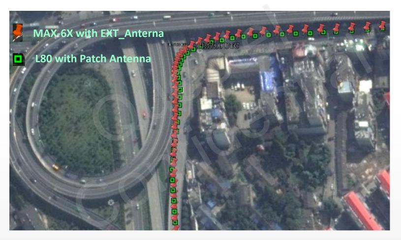
When driving across overpass and making a turn, L80 module with Patch Antenna and U company module with EXT Antenna can capture almost same accurate tracking data.
