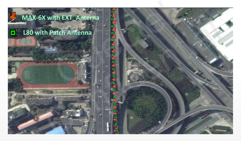
When driving under the overpass, L80 module shows its excellent performance.
