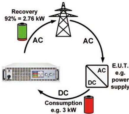
For the operation of these feeding back loads in terms of power generation it might be required to install an additional supervision unit (AIU, ENS), according to provisions of the local energy supplying companies.
